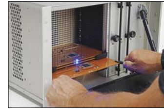
Installing an output expansion switch blade
